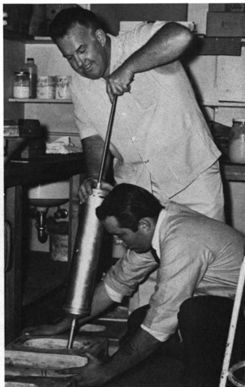
Burman and Chambers inject foam latex into the ape appliance molds. These will be baked at high temperatures in ovens. (© Apjac Productions, Inc. and Twentieth Century-Fox Film Corporation)
